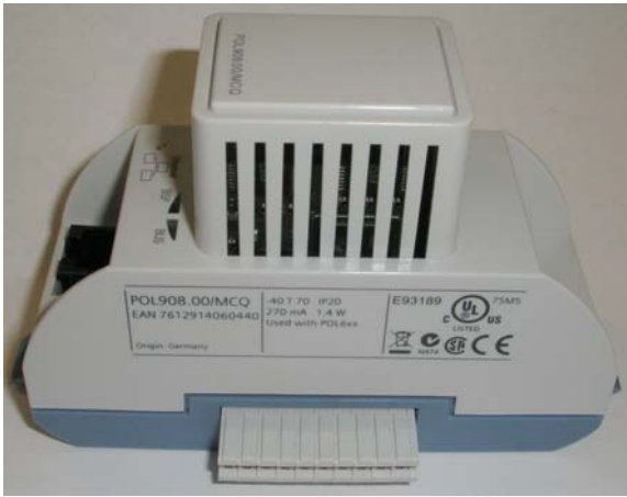
Figure 5. BACnet IP Communication Module with Board-to-Board Connector Inserted
